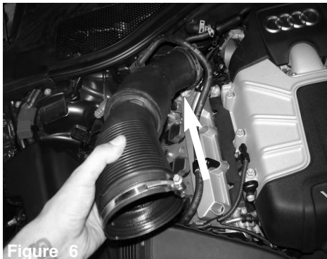
Figure 6 Pull back the vacuum line from the intake tube and remove the stock intake tube out of vehicle.
