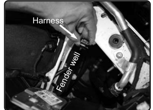
7. Disconnect the Harness located next to fender well. Pull back and remove. This will allow for more clearance when installing the air filter.
