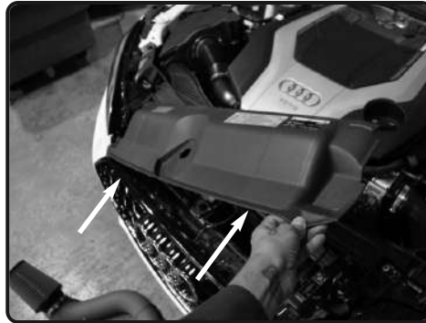
2. Push clip on hood release lever, and remove. Lift up and pull back the grille cover.
