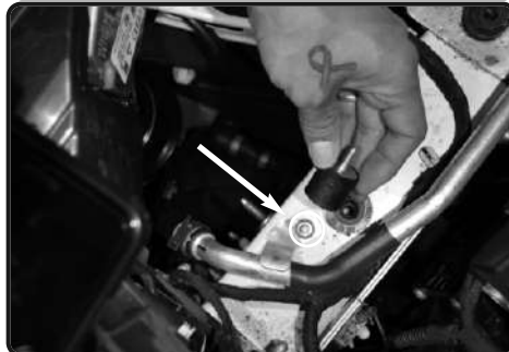
10. Locate the M6 threaded stud holding in the Air condition line on vehicle frame. Install and secure the M6 male female vibramount.
