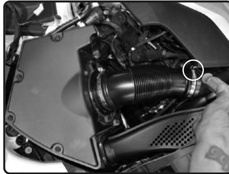
7. Loosen the clamp on the air box intake tube using 7mm nut driver.
