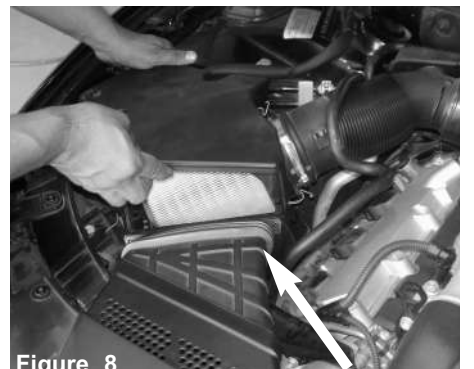
Figure 8 With all lines pulled away from the stock intake system, lift up and remove the stock intake system.
