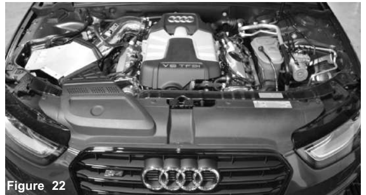
Figure 20 Install the engine cover to the top of the air box, and secure using provided coarse screws and tighten using T25 torx screw driver.
