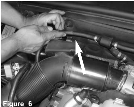
Figure 6 Pull back the vacuum line from the intake tube.
