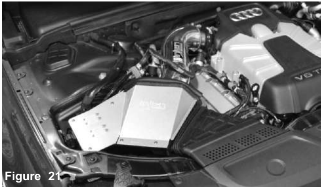
Figure 18 Rotate the intake system if needed for clearance of the filter. Position for the best fit and tighten using 8mm nut driver.
