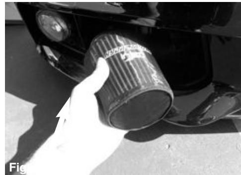
Figure 22 Install the intake tube into vehicle.
