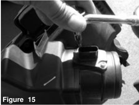
Figure 16 Carefully remove the MAF sensor.
