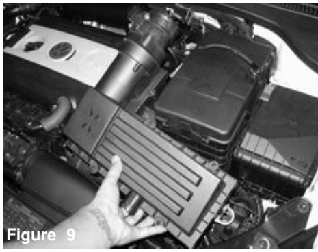
Figure 9 Pull out the complete air box assembly.
