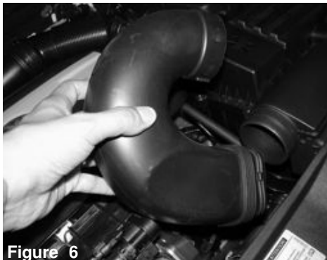
Figure 6 Pull out ram air elbow from air box.
