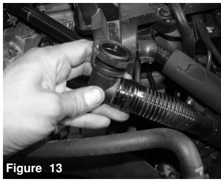
Figure 13 Rotate the smog pump fitting, if equipped, for the position of the new intake.
