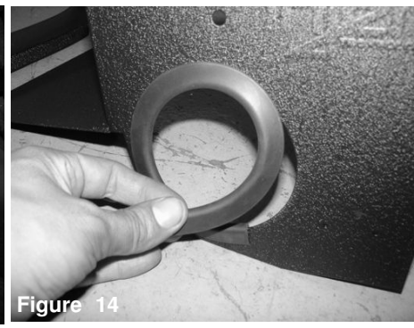
Figure 14 Attach the vinyl trim to the inside of heat shield hole cut out for the intake tube.
