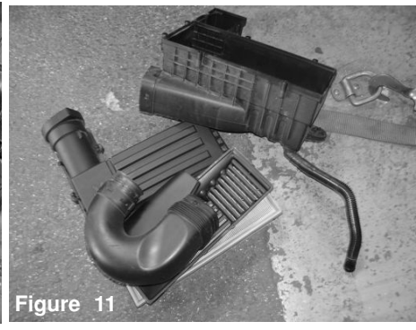
Figure 11 Complete OEM air box removed.
