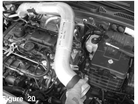
Figure 17 Install the step hose to the turbo with clamps Tighten the clamp on the turbo only using 8mm nut driver.
