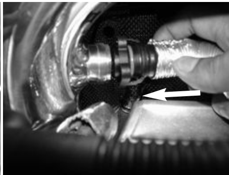
Figure 19 Secure the MAF sensor to tube using provided M4 screws and tighten using 2.5mm allen key.
