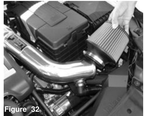
Figure 31 Make sure the power-ram is secure and tighten.
