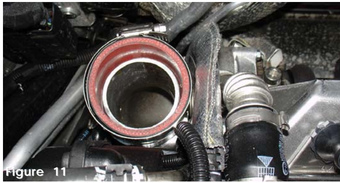
Figure 10 Press the 2 1/2" elbow over the turbo inlet until the hose is flush over the inlet.
