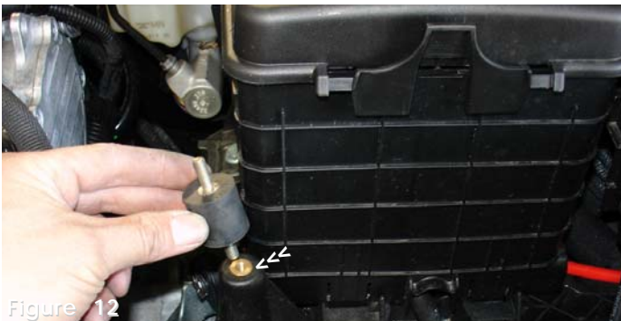
Figure 13 The vibra-mount is fully threaded into the mounting pad
