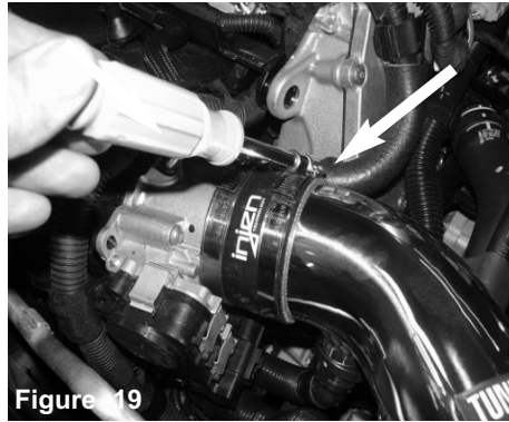
Figure 16 With light lubrication inside of the fittings on tube, secure and connect the crank case line and smog pump. Make sure you hear a click for it to be secured properly. If not equipped, use provided vinyl plug.
