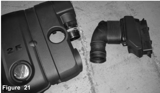
Figure 19 Position for best fit and clearance. Tighten the clamp using 8mm nut driver.
