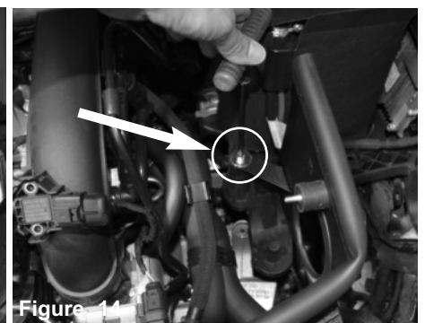
Figure 11 Install the vibramount to the heat shield and secure using provided M6 nut.
