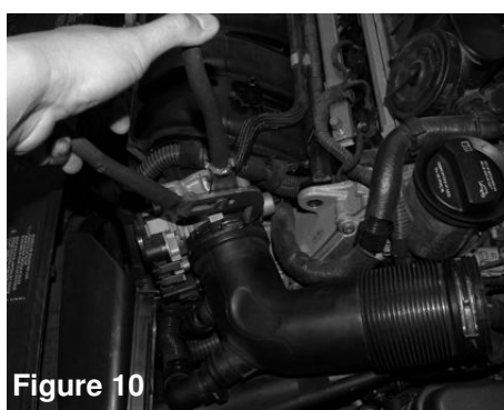
Figure 10 Use a channel lock plier to loosen the pressure clamp on the throttle body and remove the plastic air duct from the throttle body.
