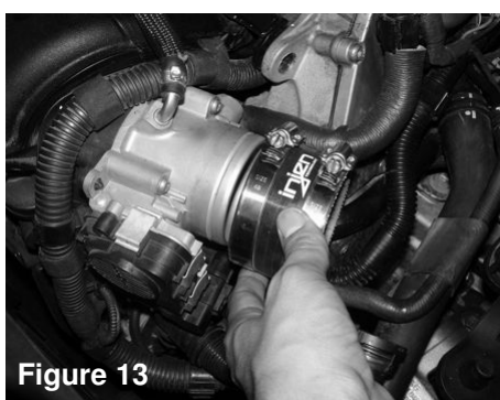
Figure 13 Place the 3.00" straight hose and 2 48 clamps onto the throttle body
