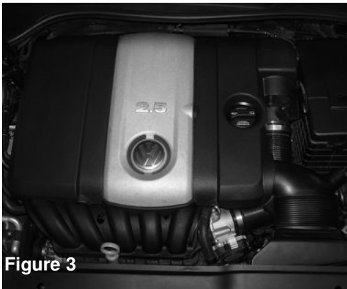
Figure 3 Picture of factory air intake system
