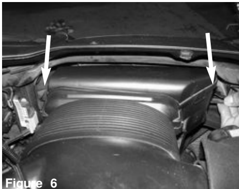
Figure 6 With T25 torx key, loosen the 2 screws holding in factory ram-air unit attached to the radiator support.
