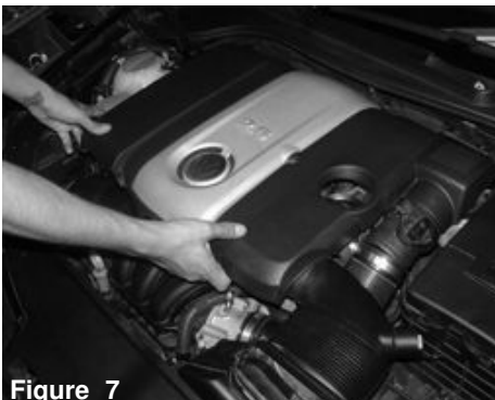
Figure 7 Carefully lift and pull up on the factory air box/engine cover and remove it from the engine.
