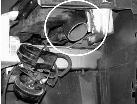
Figure 19 Place the 2.75" straight hose and two 040 clamps onto MAF sensor housing.
