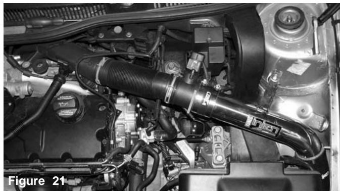
Figure 19 Now attach the 6mm vacuum hose to the welded 1/4" on the Injen intake tube. Picture shown vacuum line connected to intake tube.
