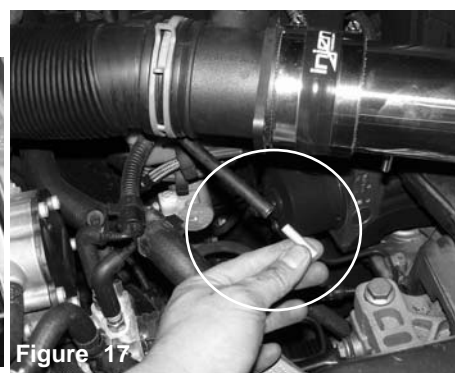
Figure 17 Place the 1 1/2" X 1/4" aluminum coupler into the vacuum hose previously removed from the air box assemble in figure 15
