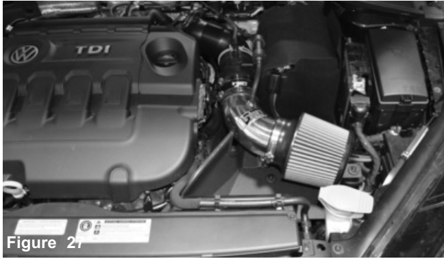
Align for best fit and tighten all clamps.
