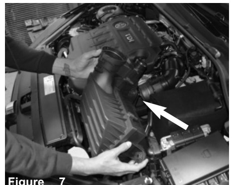
Figure 7 Lift up and remove the air box box from vehicle.
