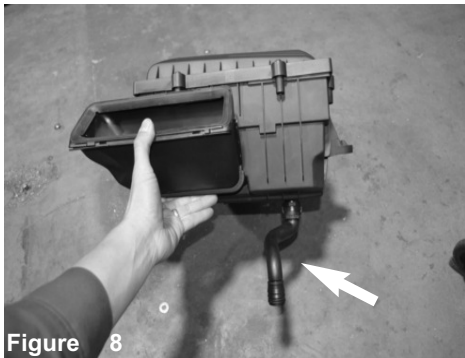
Figure 8 Now with the whole intake removed, this drain plug will not be used.
