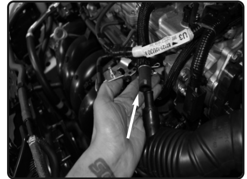
3. Disconnect the crank-case line from the intake tube.
