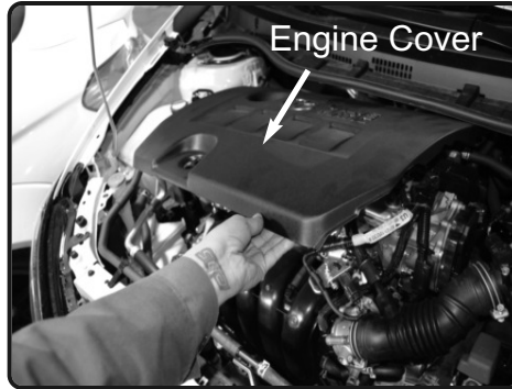
7. Carefully lift up and remove the engine cover.
