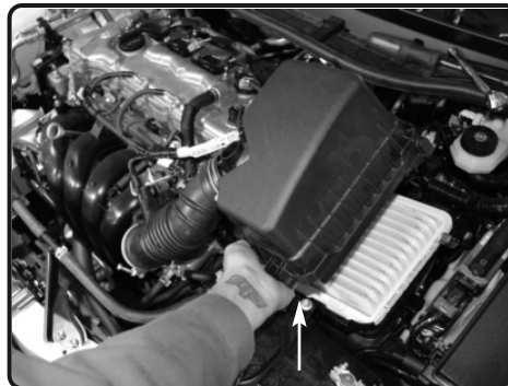
6. Loosen the clamp on throttle body. Now un-clip the upper half of the air box and remove.
