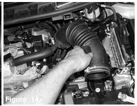
Figure 14 Remove the stock intake tube.
