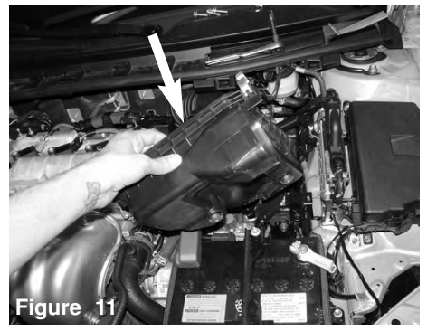
Figure 11 Remove the bottom half of air box out of vehicle.
