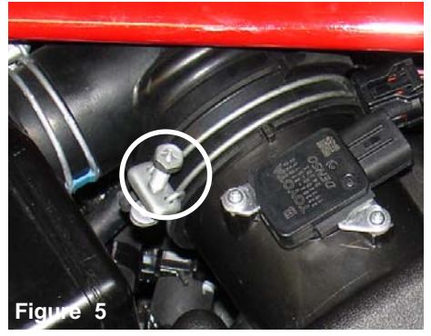
Figure 5 Loosen the hose clamp that secures the air duct to the mass air flow sensor.
