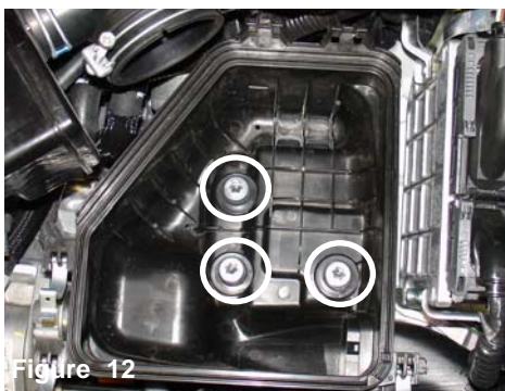
Figure 12 Loosen and remove the three m6 bolts holding the lower air box to the lower brace.
