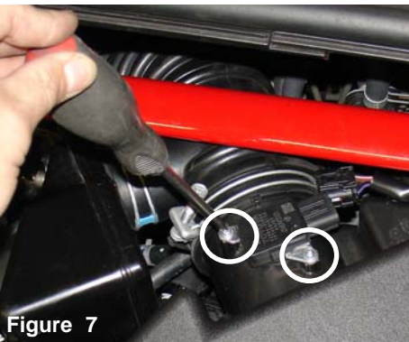
Figure 7 Unscrew and remove the two screws that fastens the mass air flow sensor to the sensor housing.
