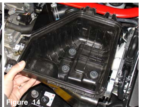
Figure 14 Once the three bolts have been removed, continue to remove the lower air box cleaner from the engine compartment.
