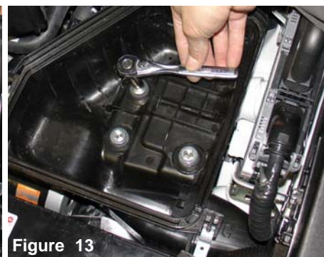
Figure 13 Use a 10mm socket to remove the m6 bolts from the air box cleaner.
