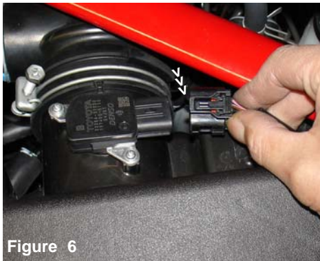
Figure 6 Disconnect the electrical sensor harness from the mass air flow sensor.
