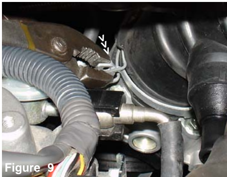
Figure 9 Depress the hose clamp located on the air duct that is connected to the throttle body.
