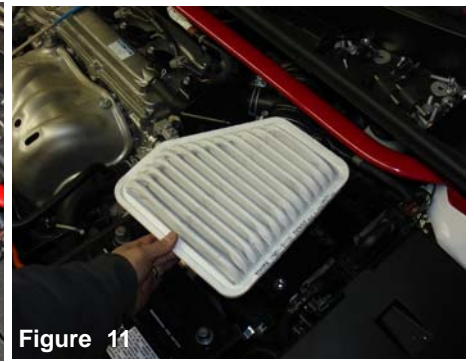
Figure 11 Once the air box top has been removed, continue to remove the white filter panel from the lower air box.
