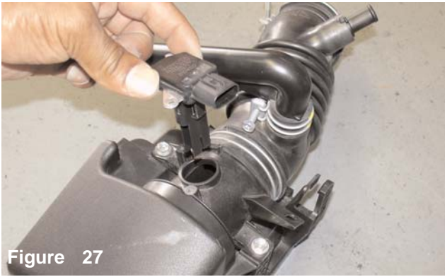
Figure 27 Once you have removed the two bolts, continue to pull the mass air flow sensor from the sensor housing.
