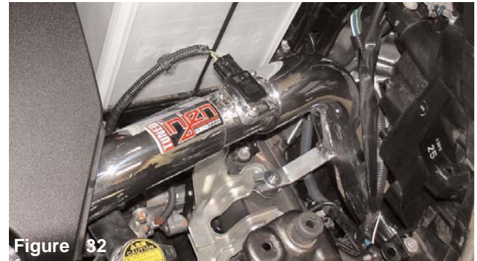
Figure 32 Congratulations! The installation is now complete. Periodically, check the alignment of the intake system for possible shifting. Shifting may cause damage to the intake that will void the warranty.
