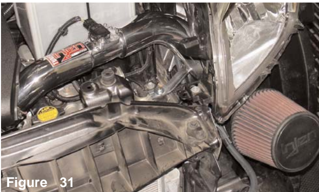
Figure 31 The entire intake system is now aligned for best possible fit. Once you have cleared the intake of any moving parts, continue to tighten all nuts, bolts and clamps. The bumper is now ready to be reinstalled.
