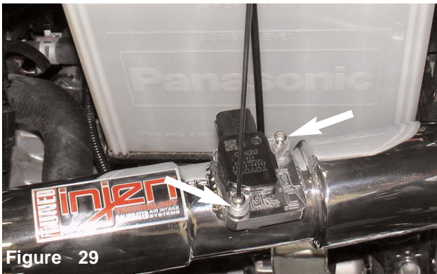
Figure 29 The two m4 x 10mm bolts in this kit are used to fasten the mass air flow sensor in place.
