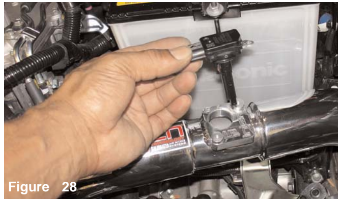
Figure 28 Insert the directional mass air flow sensor into the machined sensor adapter. A dab of light oil should be used on the O-ring to prevent kinking or tearing of the O-ring.
