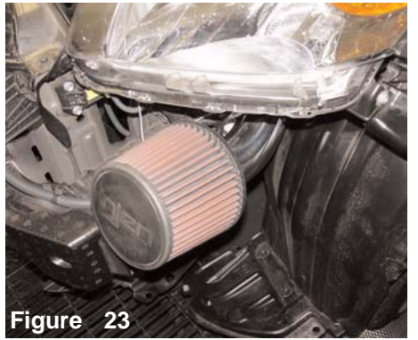
Figure 20 The m6 nut flange nut and washer are used to secure the intake to the vibra-mount.
