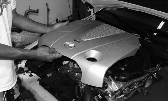
Pull the engine cover from the intake manifold by firmly pulling in a upward motion.
