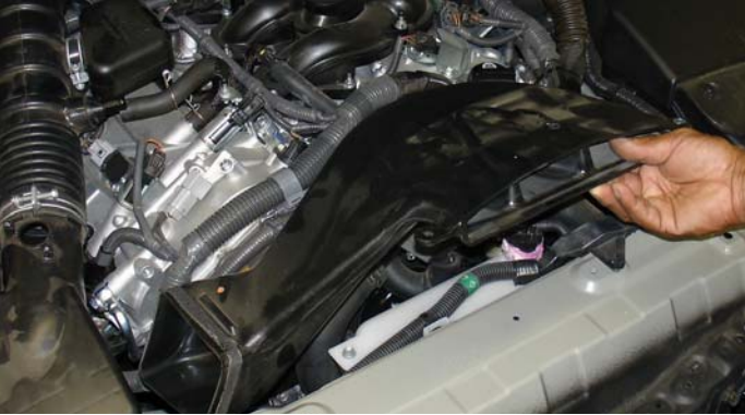
The front air scoop is now removed from its current location for now.
