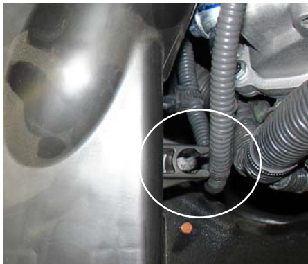
Here is a close up of the sensor harness removed from the air box clip.
