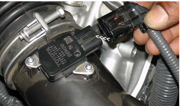
Disconnect the electrical sensor connector from the MAFS.
