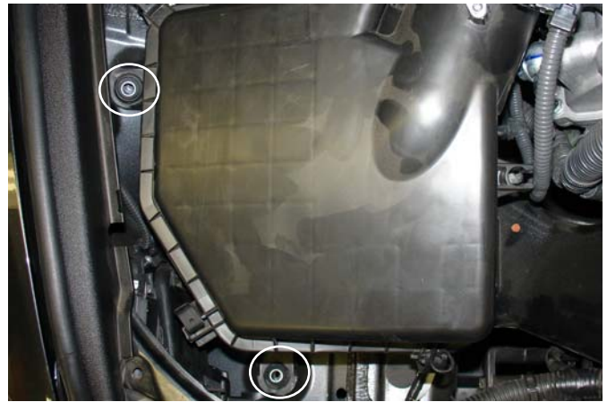
Loosen and remove the two bolts that secure the air box cleaner over the grommets.
