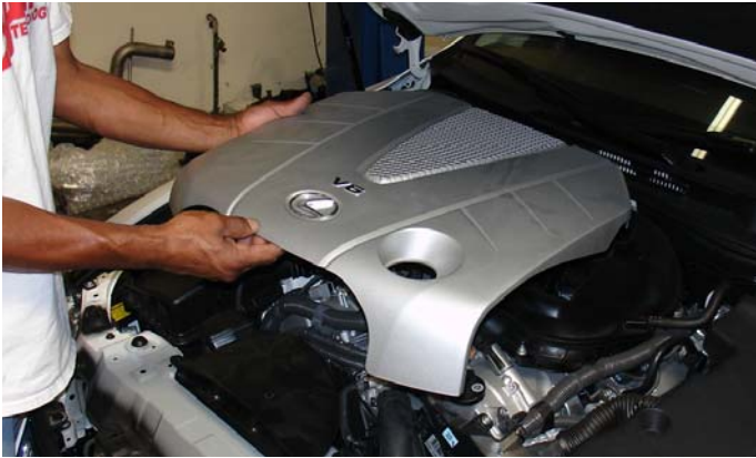
Pull the engine cover from the intake manifold by firmly pulling in an upward motion.
