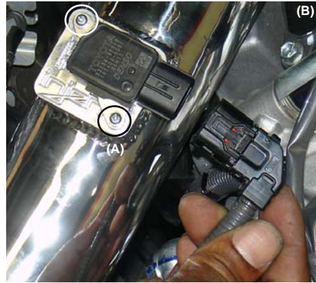
Use the stock screws to secure the MAFS in the sensor adapter (A). Firmly press the electrical sensor connector into the MAFS until it clicks in place (B).
