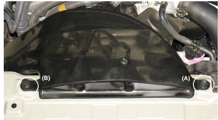
Loosen and remove one bolt (A) depress and pull the last remaining plastic clip (B) now holding the air scoop in place.
