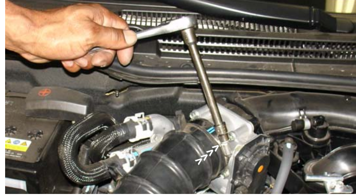
Loosen the only remaining metal clamp which secures the air duct to the throttle body as shown above.
