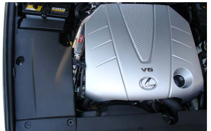
Once the intake has been fitted for a perfect fit, continue to replace the plastic air intake scoop, passenger side accessory cover and the engine cover.
