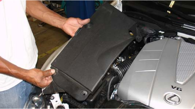
Now, continue to remove the side accessory cover which lays over the air intake box cleaner.
