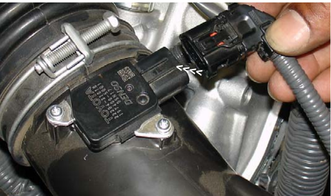
Disconnect the electrical sensor connector from the MAFS.
