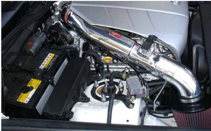
Align the entire intake for the best possible fit. Be sure the intake does not rub or hit any moving parts in the engine compartment, once you have checked the entire intake, continue to tighten all nuts, bolts and clamps.
