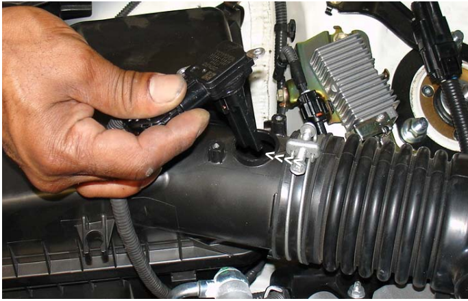
Remove the MAFS from the sensor housing as shown above. Set the MAFS to one side to be installed later in the instructions.
