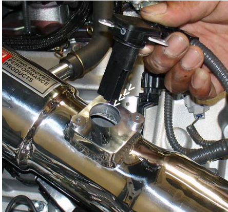
Prior to inserting the MAFS into the machined adapter, use a light weight oil around the O-ring then press the MAFS sensor into the open hole.
