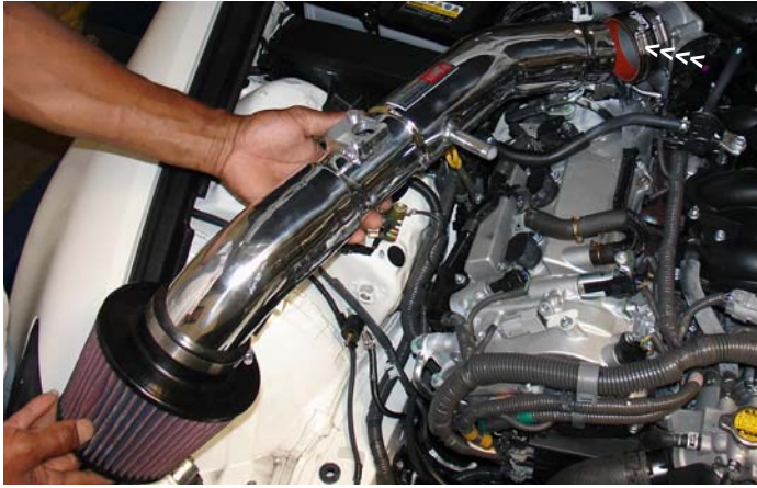
Insert the assembled air filter and intake into the engine compartment. Press the top end of the intake into the 3" throttle body hose, align the intake bracket to the vibra-mount stud and semi-tighten the clamp.
