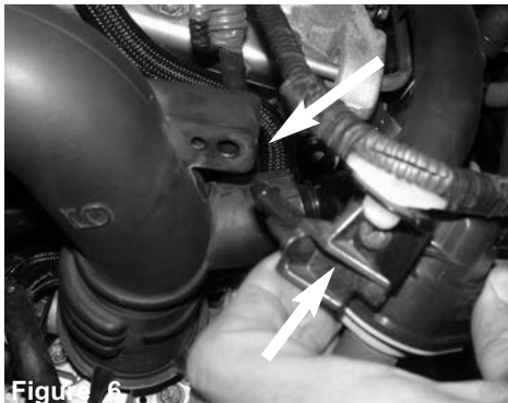
Figure 6 Pull back the VSV valve from the intake tube.
