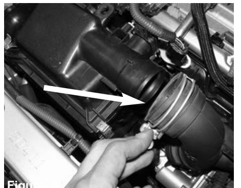
Figure 8 Pull back the intake tube from the upper part of the air box.
