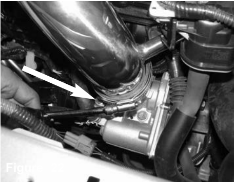
Figure 21 Connect the crank case line to the fitting and secure.
