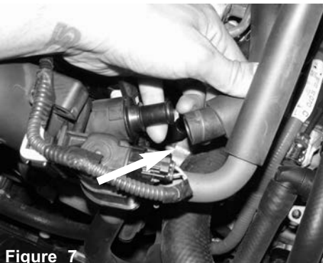
Figure 7 Pull back the crank case line from the intake tube fitting.
