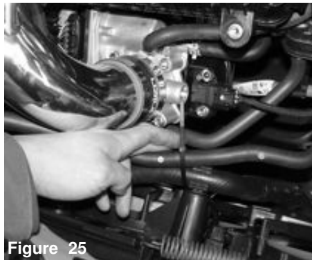
Figure 25 Zip tie the loose coolant line that was originally attached to the factory airbox.
