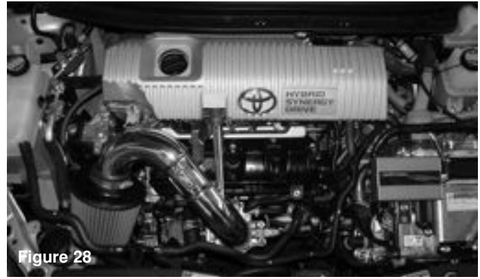
Figure 28 Congratulations! You have just completed the installation of this intake system. Periodically, check the alignment of the intake, normal wear and tear can cause nuts and bolts to come loose. Failure to check the alignment and adjust the intake can cause damage that will void the warranty.
