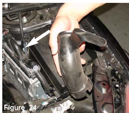
Figure 21 Once you have popped the plastic tab, continue to remove the entire plastic clip.
