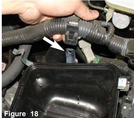
Figure 15 The upper air box is detached from the lower air box and air intake duct is removed from the throttle body.
