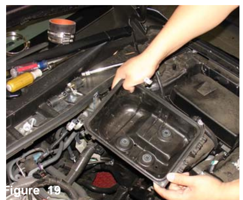
Figure 16 The stock filter panel is removed from the lower air box.
