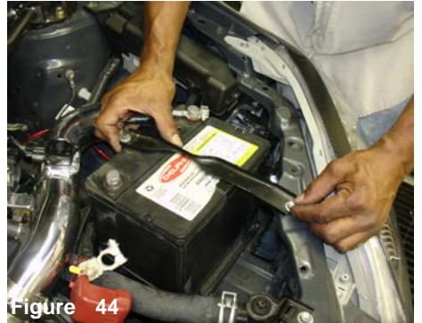
Figure 41 Once you have installed the intake, continue to re-install the battery back to its original location.
