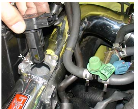
Insert the mass air flow sensor into the machined sensor adapter welded to the intake. Use the stock screws to secure the the sensor to the sensor adapter.
