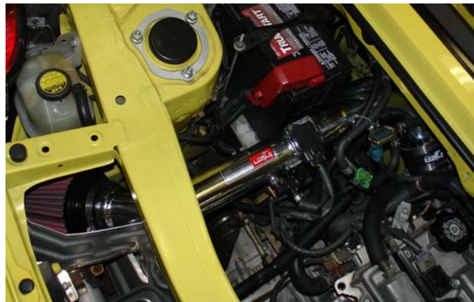
Align the entire intake for best possible fit. Once the intake has been properly fitted, continue to tighten all nuts and clamps.
