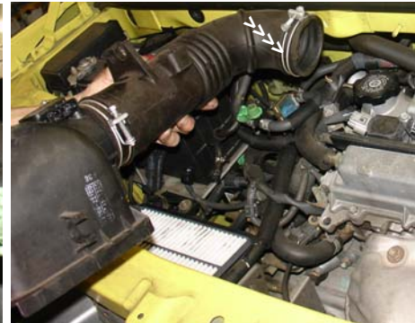
Loosen the throttle body clamp on the air intake duct and unlock the clamps surrounding the air intake box. Separate and remove the top section of the air box.
