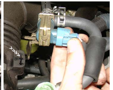
The vacuum switching valve is pulled from the holster that is built into the rubber intake duct.
