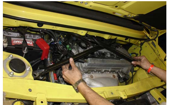
Reinstall the stabilizing bar to all its mounting points and tighten all nuts and bolts. Congratulations! You have just completed to installation of the Worlds first tuned intake system.
