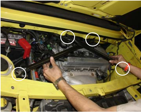
To make this installation easier, the stabilizer bar will have to be removed as shown above.
