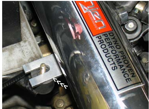
The intake bracket is aligned to the vibra-mount. Make sure that the bracket sits flush over the vibra-mount prior to fastening the bracket to the vibra-mount.
