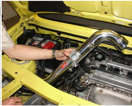
The intake is now lowered into the engine compartment to be positioned in place.
