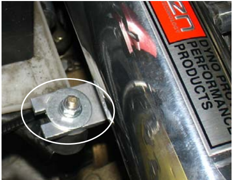
Use the m6 flange nut and fender washer to fasten the intake to the vibra-mount as shown above.
