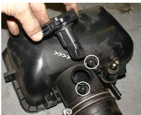
Unscrew the two screws holding the mass air flow sensor to the sensor housing.
