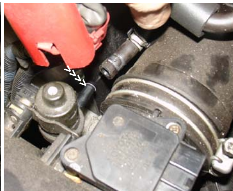
The OBD sensor vacuum hose is removed from the sensor port.
