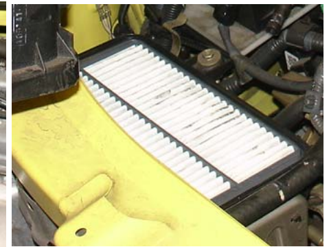
Remove the panel filter from the bottom section of the air box.
