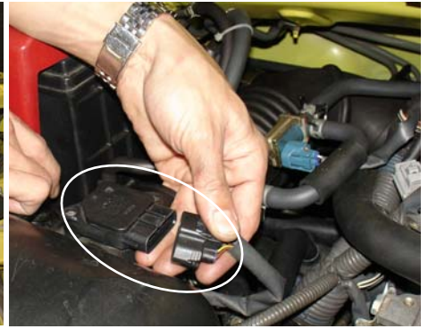
The harness clip is disconnected from the mass air flow sensor.
