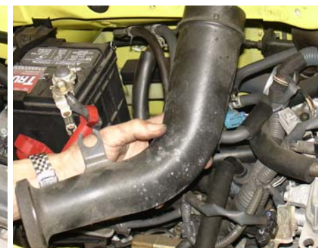
For the installation the air intake resonator is no longer required for this application.
