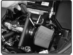
**19.** Install and tighten filter using 8mm nut driver.
