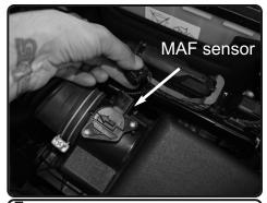
7. Disconnect the MAF sensor harness and pull harness cable from the air box.
