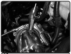
**16.** Now attach the crank case line to the intake fitting. Secure using the OEM clamp.
