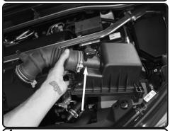
**4.** Now un-clip the upper part of the air box assembly. Lift up and remove from the vehicle.
