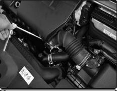
**3.** Loosen the clamp on the throttle body using 10mm socket or wrench.
