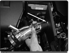
**14.** Attach the step hose with clamps to the intake tube. Install the intake tube assembly into the vehicle and position.
