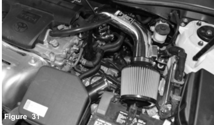
Figure 31 Congratulations! You have just completed the installation of this intake system. Periodically, check the alignment of the intake, normal wear and tear can cause nuts and bolts to come loose.
