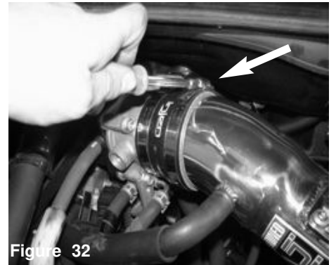
Figure 29 Install the intake tube assembly into the vehicle and position to the throttle body, and position the bracket to the vibra mount.
