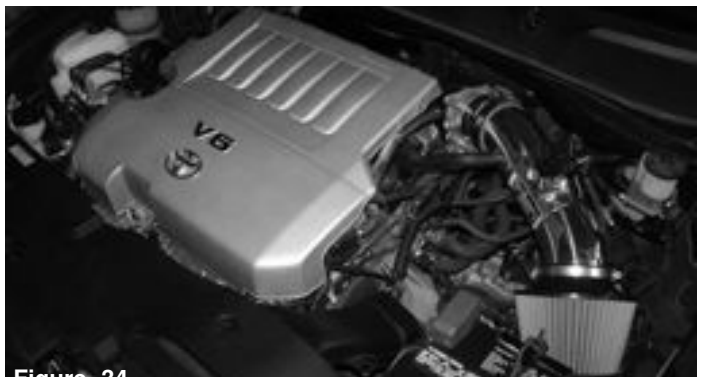
Figure 31 Connect the crank case line to the fitting on intake. Connect the vacuum line from step 12 to the smaller fitting on new injen intake tube.
