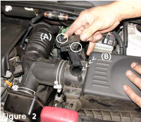
Figure 2 Unclip the harness clip from the electrical mass air flow sensor, unscrew the two screws on the sensor (A) and pull the air mass sensor out of the sensor housing (B).
