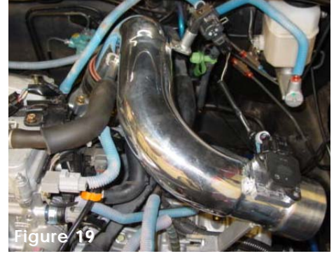
Figure 19 The primary intake is installed and ready for the filter.
