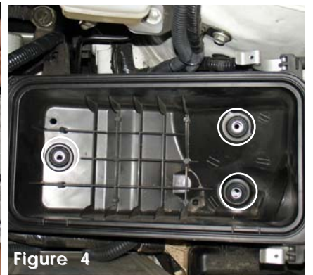
Figure 4 Unscrew the three m6 bolts from the lower air box cleaner. Note: This lower air box cleaner is used for illustration purposes only.
