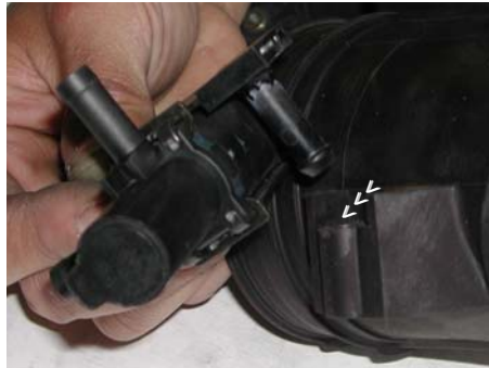
Figure 15 Remove the carbon canister from the rubber intake duct saddle.
