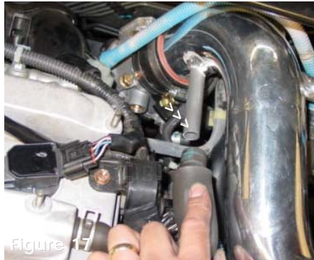
Figure 17 Press the stock breather line over the long intake port.
