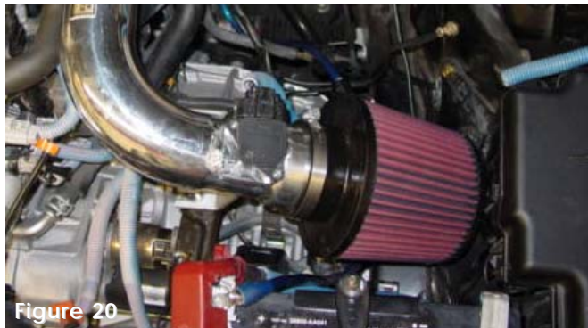
Figure 20 Press the filter over the intake end and tighten the filter clamp. Align the entire intake for best possible fit. Once the intake has been cleared from any moving objects, continue to tighten all nuts, bolts and clamps.
