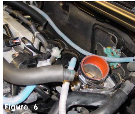
Figure 6 Press the 2 3/4" straight hose over the throttle body and use two power bands, tighten the clamp on the throttle body side for now.
