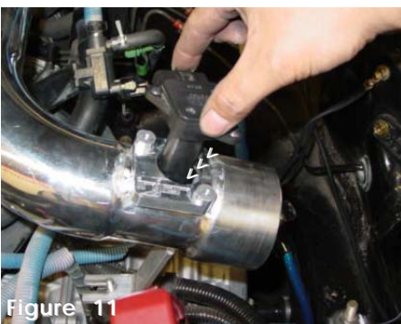
Figure 11 Insert the mass air flow sensor into the machined intake adapter. Use a dab of light oil on the sensor O-ring prior to pressing the sensor into the adapter.
