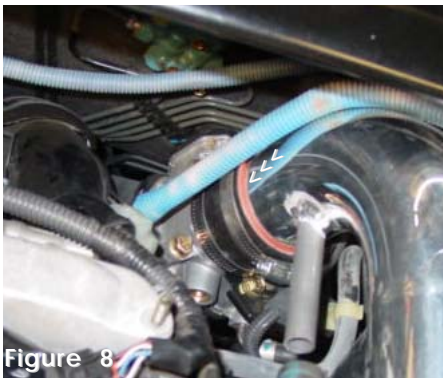
Figure 8 Place the intake in the engine compartment and insert the top end in the throttle body hose.
