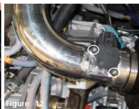
Figure 12 Use the stock screws to secure the sensor to the machined adapter.
