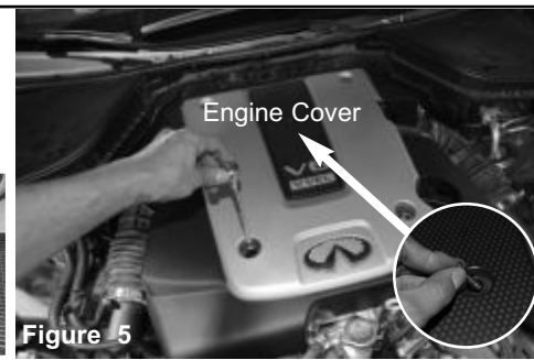
Figure 5: Remove the 3 bolts and 2 nuts holding in the engine cover. Lift up and remove the engine cover.
