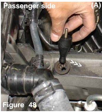
Align the composite stand-off over the stock grommet (A) push down on the stand-off until it is fully inserted into the grommet (B)..
