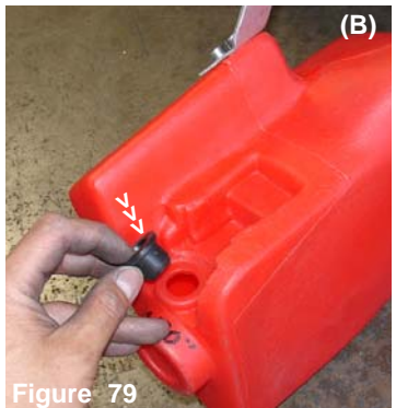
Figure 78 Use the last of the m6 x 12mm bolts to fasten the bracket to the reservoir bottle as shown in figure (A). The grommet that was removed from the stock reservoir bottle is now inserted into the new reservoir bottle (B).
