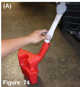
Figure 74 The top spout is aligned to the spout on the reservoir tank (A). The top bracket is aligned over the press nuts on the top of the reservoir bottle (B). Note: The stock level sensor indicator will not be used for this installation because of the difficulty of cutting out and removing the sensor.
