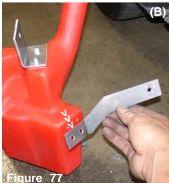
Figure 76 Use the m6 x 12mm bolts in this kit to fasten the bracket to the reservoir bottle (A). The horizontal long bracket is now aligned to the side m6 press nuts (B)
