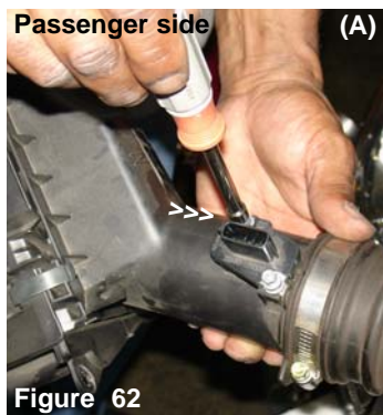
Removing the bolts from the mass air flow sensors: Use an 8mm nut driver to remove the 4mm bolts from the mass air flow sensors as shown above. Once you have removed the bolts, continue to pull the mass air flow sensor from the sensor housing, repeat the same steps on the driver side sensor housing.
