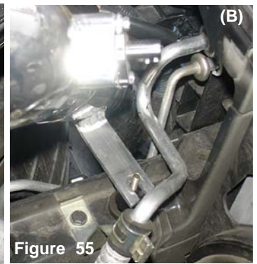
The intake bracket is sitting firm over the stand-off (A) the same is repeated on the driver side, the intake bracket is sitting firm over the stand-off (B).
