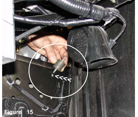
Figure 12 Pull the resonator box out of the grommet pins used by the resonator box. The resonator box will not be used as part of this installation.
