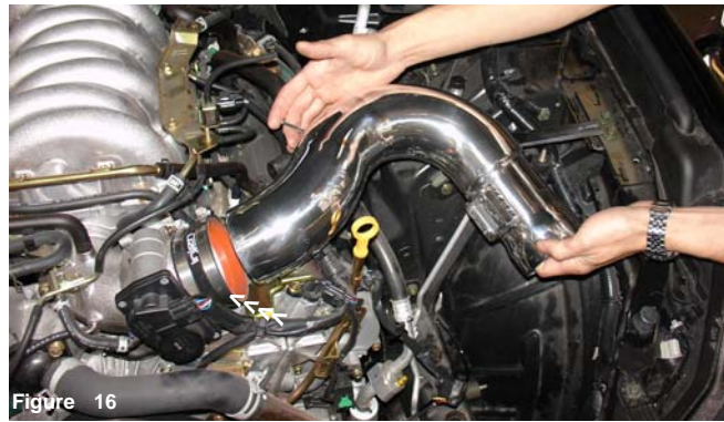
Figure 13 Press the straight hose over the throttle body and use two power bands. Once the hose has been placed over the throttle body, use a nut driver to tighten the power band on the throttle body side.
