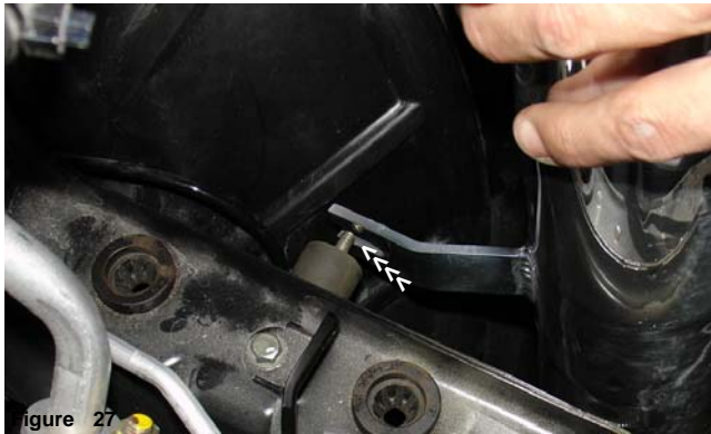
Figure 27 align and set the intake bracket over the vibra-mount stud. Press the top end of the secondary intake into the hose located on the primary intake.
