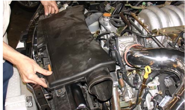
Figure 28 Once the Primary and secondary intakes have been aligned continue to semi-tighten the power-band (A). Use the m6 flange nut and fender washer to secure the intake to the vibra-mount stud (B).
