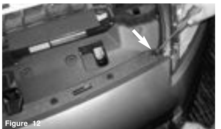
Figure 12 Pop all 7 plastic tabs and remove clips located on the bumper lip.
