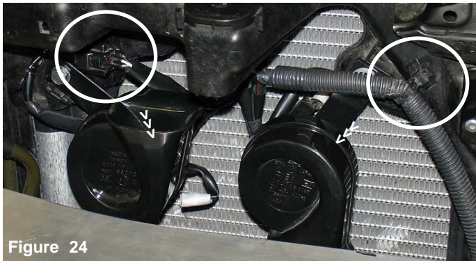
Figure 24 Stock horns to be removed and relocated. Circled above are the harness clip and wire loom that need to be removed from the crossmember, this will allow the harness and horns to be relocated into the lower bumper area.
