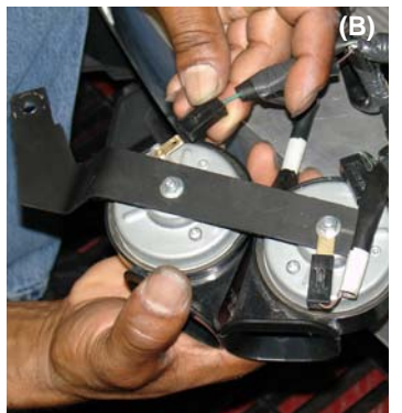
Figure 29 The second horn is aligned and attached to the top of the new bracket, the nut is used to secure the horn in place (A). The electrical wires are reconnected as shown above (B).
