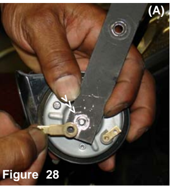
Figure 28 The first horn is aligned and attached to the new bracket, the copper connectors are re-attached prior to securing it with the nut (A). The copper connector is re-attached and the electrical wires are reconnected as shown above (B).
