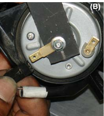
Figure 28 The first horn is aligned and attached to the new bracket, the copper connectors are re-attached prior to securing it with the nut (A). The copper connector is re-attached and the electrical wires are reconnected as shown above (B).
