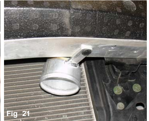
The plastic clip is shown here locating the intake to the bottom of the bumper reinforcement.
