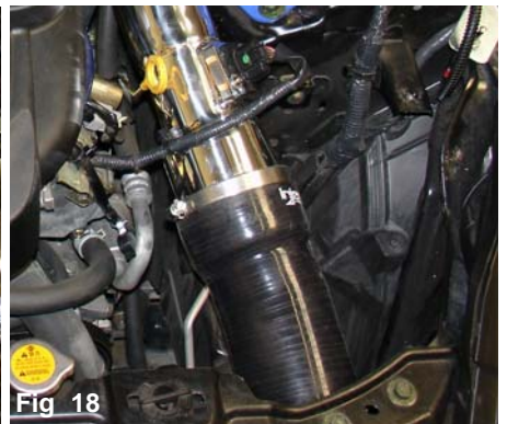
Fig 18 The 3 1/2" top end of the hose is pressed over the primary end of the intake. Use one .412 large power-band to secure the hose in place.
