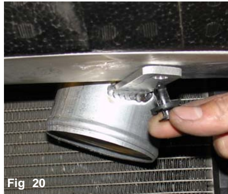
Line up the pre-tapped hole on the bumper reinforcement to the intake bracket. Use the stock plastic clip to secure the intake in place.
