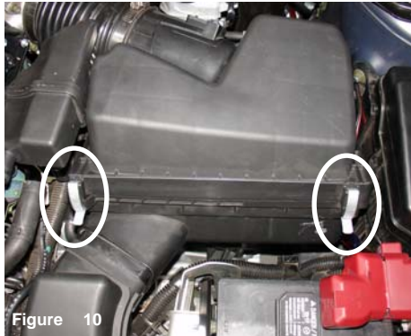
Figure 10 These are the two metal clips that are to be removed from the air box. These two clips connects the top air box to the lower air box.
