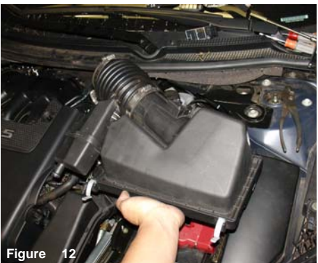
Figure 12 Once the metal clips have been unsnapped, continue to remove the top air box along with the CCV box and air intake duct.
