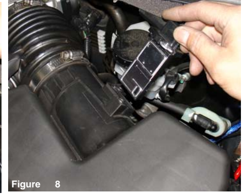
Figure 8 Once you have removed the two bolts, continue to pull the mass air flow sensor out of the sensor housing. This mass air flow sensor will be used later in the installation.
