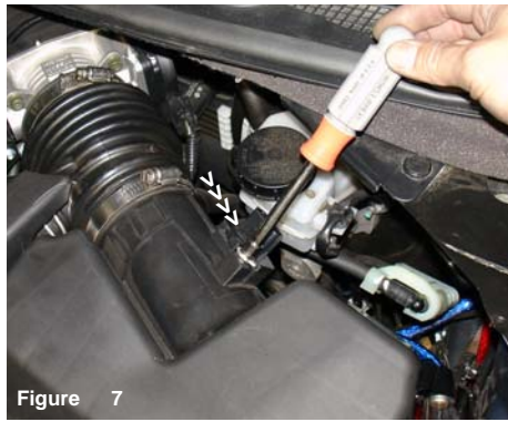
Figure 7 Unscrew the two bolts that secures the mass air flow sensor to the sensor housing.
