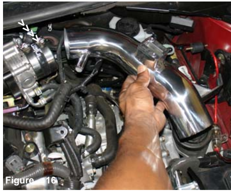
Figure 16 Lower the air intake into the engine compartment and press the upper end into the throttle body hose.
