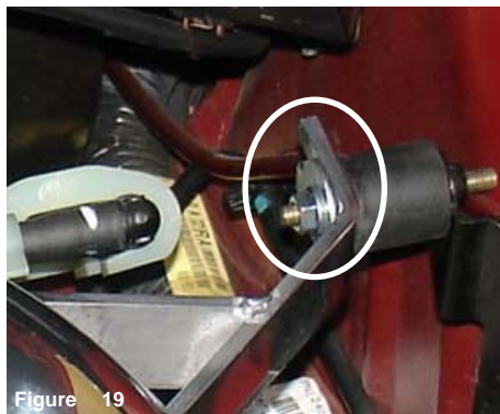
Figure 19 The m6 flange nut and fender washer is used to fasten the air intake to the vibra-mount stud.
