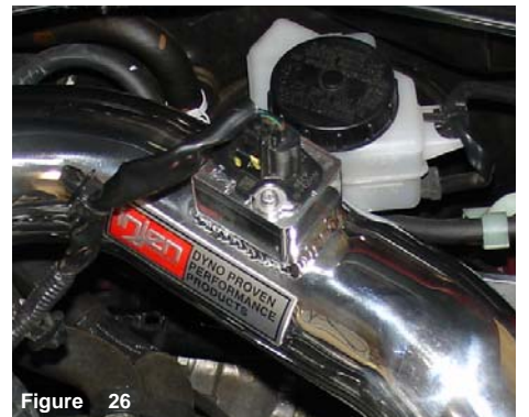
Figure 26 The electrical sensor harness is now reconnected to the mass air flow sensor.
