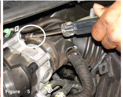
Figure 5 use an 8mm nut driver or screwdriver to loosen the throttle body clamp.
