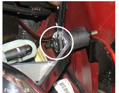
Figure 20 The m6 flange nut and fender washer is now securing the air intake. Do not over tighten the m6 nut until the assembled filter and heat shield has been installed.
