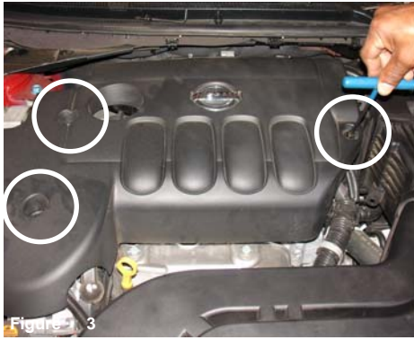
Figure 3 Using an allen wrench, remove all three m6 bolts from the engine cover.
