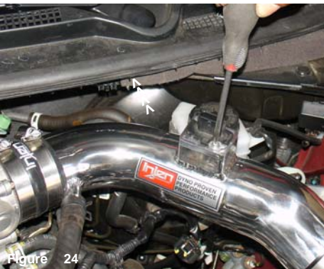
Figure 24 Once the mass air flow sensor is sitting flush with the billet sensor adapter, continue to use the stock bolts to secure the air sensor in place.
