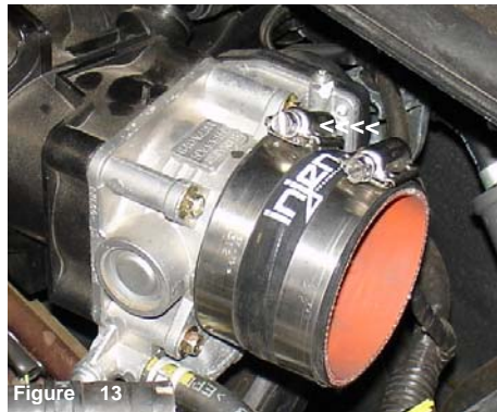
Figure 13 Press the 2 3/4" straight hose over the throttle body and use two power band. The power band on the throttle body is tightened at this point.
