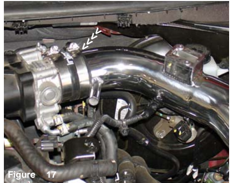
Figure 17 The intake is now lowered into the engine compartment and into the throttle body hose.
