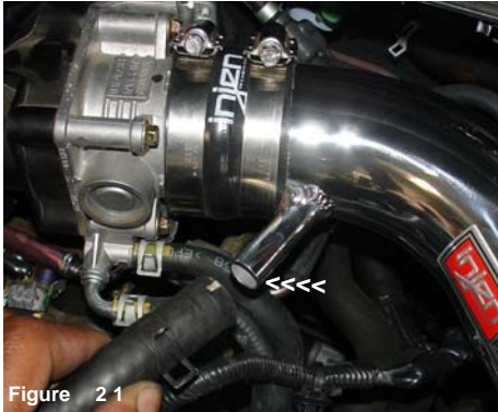
Figure 21 Align the crankcase vent hose to the intake port as shown above.
