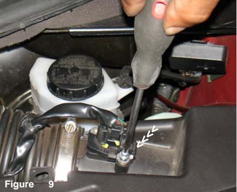
Figure 9 Unscrew the two bolts that secures the mass air flow sensor to the sensor housing.
