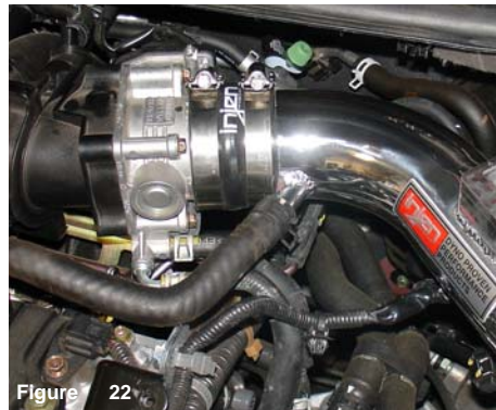
Figure 22 Once the crankcase vent hose has been pressed into the intake port, continue to reuse the wire tension clamp to secure the hose in place.
