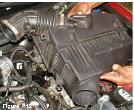
Figure 12 Once bolts and clamps have been removed or loosened, continue to pull the entire air intake box and air intake tract from the engine compartment.
