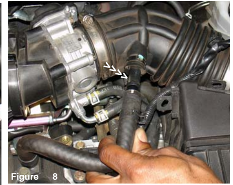
Figure 8 Once the tension clamp is pulled away, continue to pull the hose away from the CCV box.
