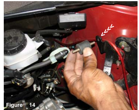
Figure 14 align the vibra-mount to the bracket located to the side of the strut tower mount.
