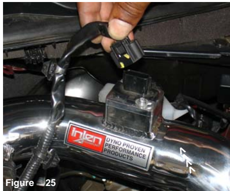
Figure 25 Take the electrical sensor harness and press it over the mass air flow sensor. Press all the way down until you hear the clip snap the two together.
