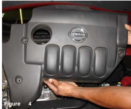
Figure 4 Once all three bolts are removed, continue to pull the engine cover from the air intake manifold and valve cover.
