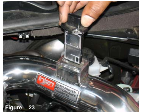
Figure 23 Insert the original mass air flow sensor into the machined billet sensor adapter. To prevent kinking of the gasket, be sure to use a light oil to moisten the gasket.
