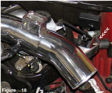
Figure 18 The intake is pressed into the throttle body hose and the intake bracket is aligned to the vibra-mount stud.
