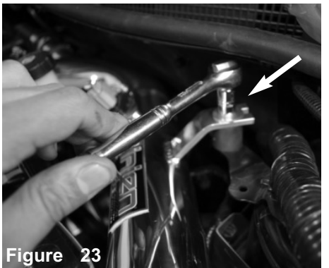
Figure 20 Install the intake tube into vehicle and position to the hump hose and the bracket to the vibramount.
