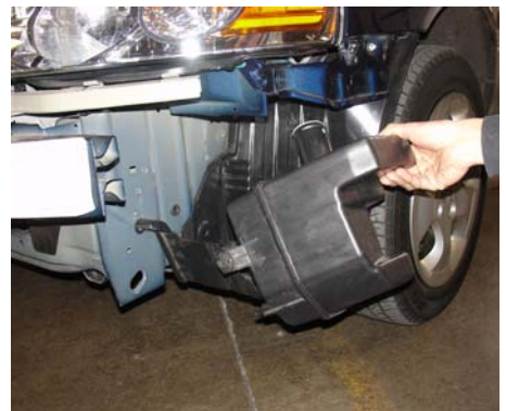
Remove any bolts from the air resonator box then continue to remove the air resonator box as shown above.
