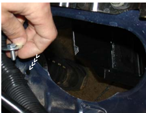
Take the m6 x m12 bolt and washer. Insert the bolt into the hole that was occupied by the plastic clip.
