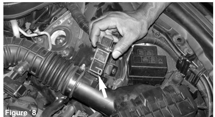
Figure 6 Depress the tab and pull the electrical harness connector from the mass air flow sensor.
