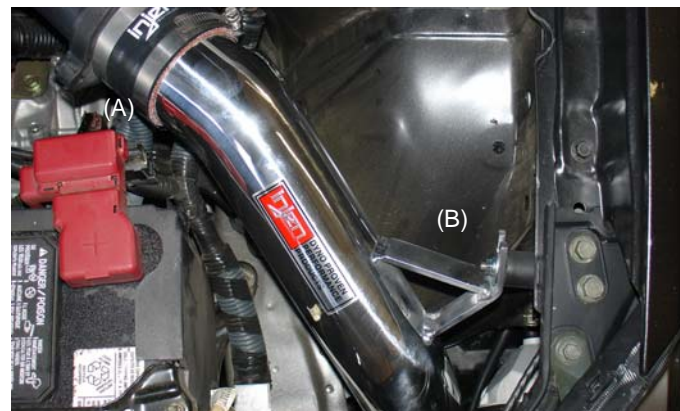
Press the top end of the intake into the primary hose (A). Align intake bracket to the vibra-mount stud (B). Adjust secondary intake and semi-tighten clamp(A). Place fender washer and m6 flange nut over the vibra-mount stud without tightening yet (B).
