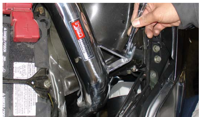
Align entire assembled intake and use a Ratchet or nut driver to tighten the m6 flange nut to the vibra-mount.
