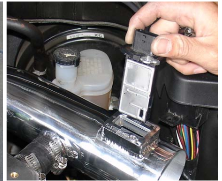
Take the MAF sensor and insert it into the machined MAF sensor adapter.
