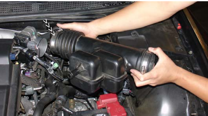
Loosen clamp at the throttle body and remove the air intake duct. At this point, it will be necessary to remove the front bumper. Remove 9 clips on top of the bumper, two 10mm screws on each side of the bumper, four additional sheet screws and 5 plastic clips.
