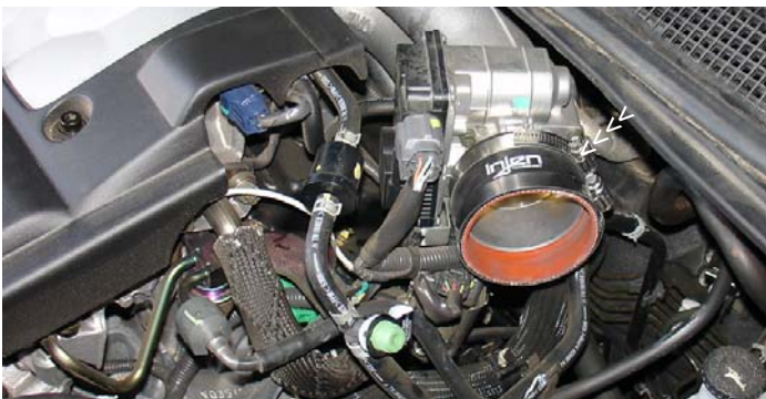
Press the 3 1/8" straight hose over the throttle body and use two clamps. Tighten the clamp located over the throttle body at this point.
