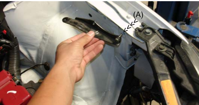
The bracket used to hold the stock air box in place will no longer be used. Remove the stock bracket to make room for the m6 vibra-mount. New location for the vibra-mount (A).
