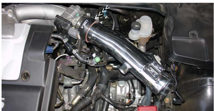
Insert the top end of the intake into the throttle body hose. Semi-tighten the clamp just enough to hold the intake in place.
