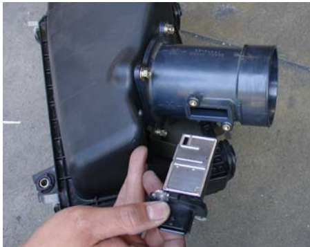
Use the torx bit in this kit to unbolt screws from the MAF sensor. Carefully, remove the MAF sensor from MAF sensor housing.
