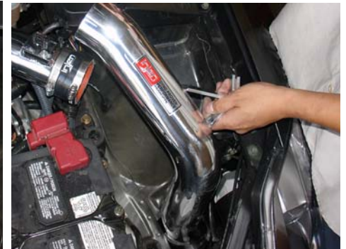
Carefully, lower the secondary intake into the resonator opening and into the bumper corner.
