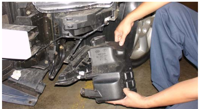
Once the bumper has been removed continue to disconnect and remove the plastic air intake resonator box.
