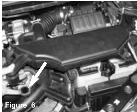
Figure 3 Prior to starting the installation, remove the 2 m6 bolts holding the engine cover in place
