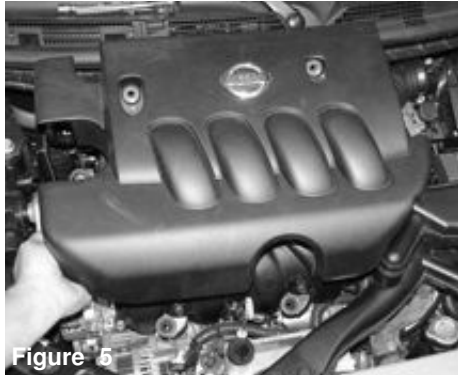
Figure 3 Prior to starting the installation, remove the 2 m6 bolts holding the engine cover in place
