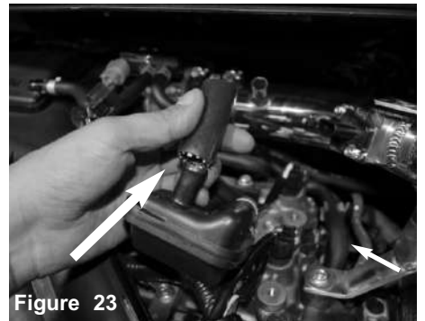
Figure 20 Install the intake tube. Position the intake tube to the hose and bracket to vibramount.
