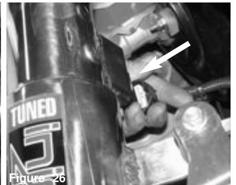
Figure 23 1) Secure the top of the vibra mount using provided M6 nut. 2) Secure the bottom of the vibra mount using provided M6 nut and washer.
