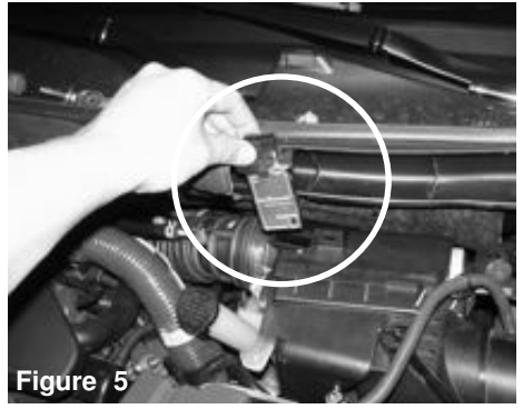
Figure 5 : Pull the MAF sensor out of the factory air box housing.
