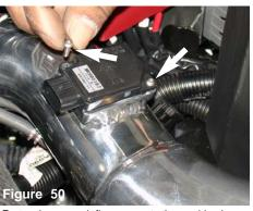
Fasten the mass air flow sensor to the machined adapter with the m4 x 10mm bolts.
