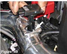
Carefully insert the mass air flow sensor into the machined sensor adapter. We recommend you apply a small of amount of light oil on the O-ring to prevent any kinking or tearing.
