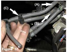
Both stock lines connected to the solenoid are removed from ports (A) and (B). The two into one check valve will no longer be used (C).
