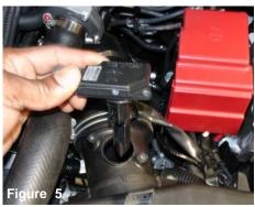
Once you have removed the stock bolts, continue to pull the mass air flow sensor from the sensor housing.
