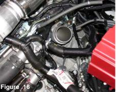
The air box cleaner and air intake duct have been removed and the turbo inlet is now exposed.
