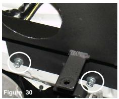
The heat shield slots are inserted between the bolt head and car frame, once the heat shield brackets have been aligned and fastened, continue to tighten the 12mm bolts
