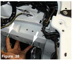
The bracket bolts that were removed in figure 24 are used in this picture, leave enough gap to slide the heat shield slots over the bolts.
