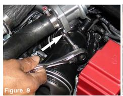
Loosen the lower clamp that secures the BOV to the port on the air intake duct.
