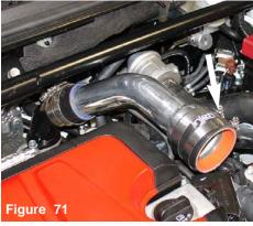
Once the hose has been installed, continue to tighten the clamp over the tubing.
