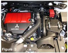
Stock air intake cleaner and upper intercooler piping shown in this picture
