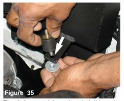
The m6 vibra-mount is inserted into the hole located on the heat shield bracket. The m6 flange nut and fender washer are used to fasten the vibra-mount to the bracket.
