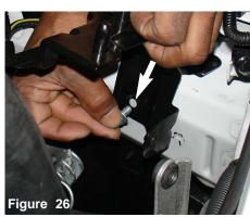
The 4th and final 12mm bolt is loosened and removed from the bottom of the air box bracket. The bolt is replaced to hold the new heat shield.
