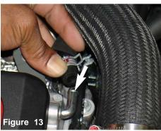
Disconnect the 10mm breather hose from the crankcase port as shown above.
