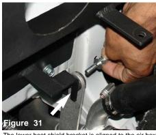
The lower heat shield bracket is aligned to the air box brace. The stock 12mm bolt is inserted into the stock air box rubber vibration mount and into the heat shield slotted bracket
