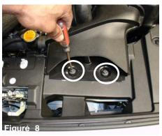
Use a flat head screw driver to pop the plastic clips from the front air scoop.
