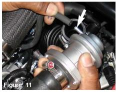
Once you have pulled the BOV from the air intake port, remove the 4mm vacuum line from the BOV port.
