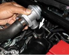
Now that the BOV clamp is loose, continue to pull the BOV from the air intake port.
