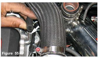
The remaining end of the 10mm crank case hose is pressed over the crank case port.
