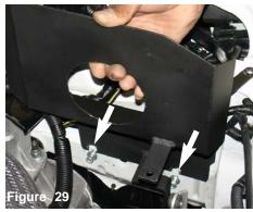
The heat shield is lowered and aligned to the two 12mm bolts.
