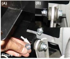
The m8 flange nut is used to secure the heat shield bracket to the air box brace (A). The m8 flange nut is tightened on the 12mm bolt (B).
