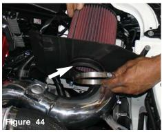
Remove the filter neck clamp from the filter, insert the filter neck into the heat shield hole and align the filter to the intake as shown above.
