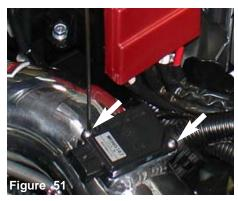
An allen wrench is used to tighten the bolts to the mass air flow sensor.
