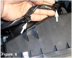
Disconnect the electrical sensor harness from the upper air box cleaner.
