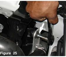
The 3rd 12mm bolt is loosened and removed from
