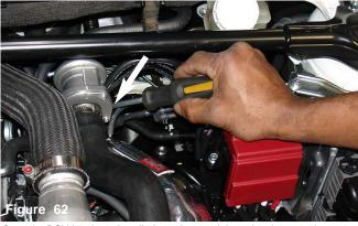
Once the BOV has been installed, continue to tighten the clamp on the straight hose.  $% \label{eq:continuous}$
