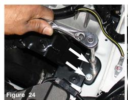
Loosen and remove the two 12mm bolts on the air box bracket. Note: These two 12mm bolts will be used later the bracket as shown above. in the instructions, see figure 28.
