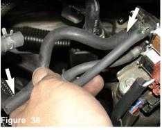
The 6" -4mm hose is pressed over the lower solenoid port.
