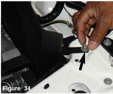
The upper heat shield bracket is aligned to the threaded hole. Once the bracket is aligned to the pre-threaded hole, continue to fasten the bracket with the stock 10mm bolt.
