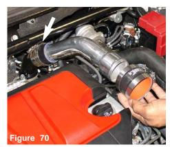
Adjust and semi-tighten the clamp on the tubing. Press the 2 1/2" hose over the opposite end of the tubing. Place two clamps over the 2 1/2" hose.
