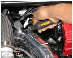
Use the 8mm press nut to tighten the clamp on the step hose.
