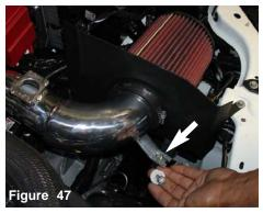
Use the m6 flange nut and fender washer to fasten the intake bracket to the vibra-stud
