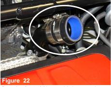
Press the 2" x 2 1/2" long straight hose over the upper intercooler inlet, use two .032 power-bands on the straight hose. Tighten the clamp on the inlet side
