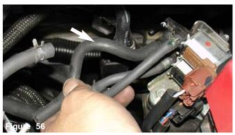
Align the lower 4mm hose over the intake port
