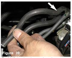
The 6 3/4" -4mm hose is pressed over the upper solenoid port as shown above.
