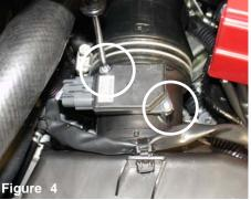
The stock bolt are removed from the mass air flow sensor as shown above.
