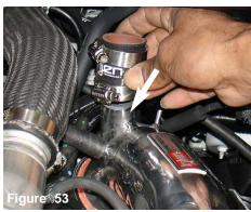
Press the 1 3/8" hose over the intake BOV port, place two small clamps on the hose, tighten the lower clamp over the BOV hose.
