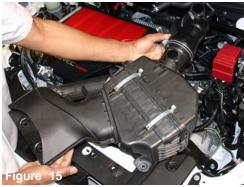
Once all clamps, bolts and clips have been loosened or removed, continue to pull the entire air box cleaner from the engine compartment.
