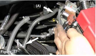
Once you have pressed the 6'-4mm hose over the lower solenoid port (A) continue to press the other end over the lower intake port (B).
