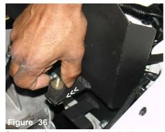
Once the m6 flange nut and fender washer have been semi-tighten under the bracket, continue to turn the vibra-mount until it is firmly tightened.
