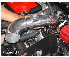
The primary intake is lowered into the engine compartment and pressed into the turbo step hose.
