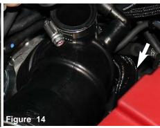
The clamp on the air intake duct that connects to the turbo inlet is loosened.
