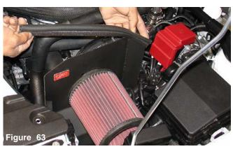
Align and press the vinyl trim over the edge of the heat shield.
