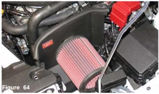
The vinyl trim is now installed over the heat shield edge.
