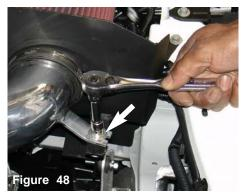
The intake bracket is tightened with a 10mm sockets and ratchet as shown above.
